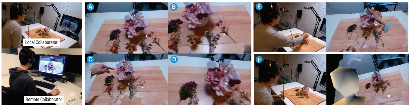
Figure 12: Demonstrating interactions during a flower arrangement session. A remote viewer observes an overview of the overall flower design (A), zooms in to closely look at these flowers on the table that are available (B), sees a local collaborator pointing at a specific flower to explain the flower (C), and the viewer changes viewing angle to see the referenced flower from a side (D). A local user then adds a flower to the existing arrangement (E) and a remote viewer sees the modified design in high fidelity, while being aware of attention of the local collaborator (F).
