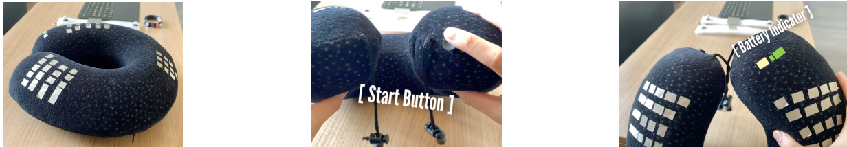
Figure 3: From left to right: prototype of the FunKey Travel Pillow, one illustrative feature of the start button, and another one of the battery indicator
