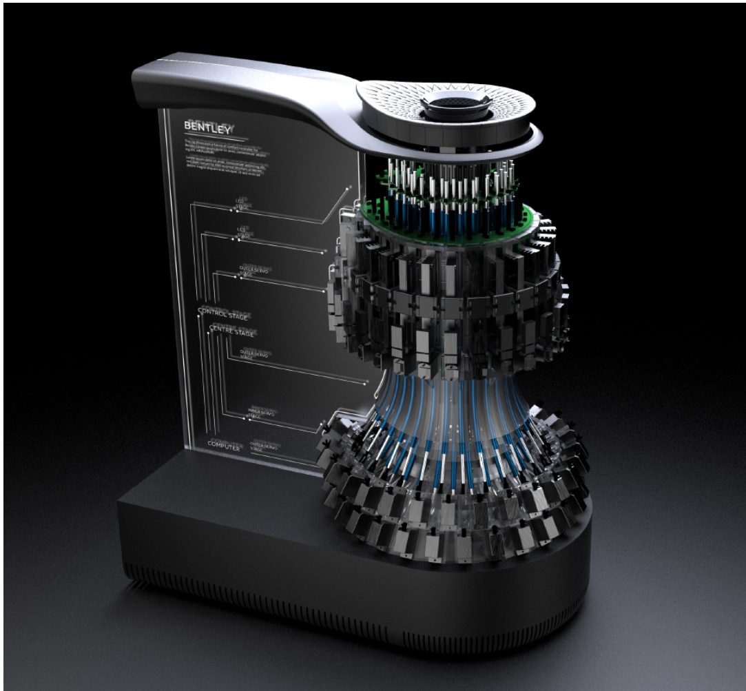
Figure 2: Rendering of research tool, the user interacts with the top surface of the unit, as each diamond shard lifts up and down, pushed and pulled by the servos on the bottom.
